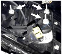
\*\* Image shows the screws from behind with fog bracket still installed.
